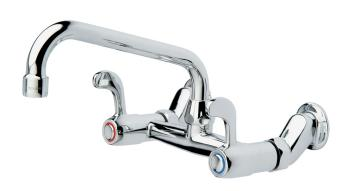
EZF1 PRODUCT CODE COLOUR/FINISHES Chrome All Pressures PRESSURE TYPE 17kPa MIN. PRESSURE MAX. PRESSURE 500kPa (As per NZ Building Code AS/NZ 3500.1) Low/Unequal 4 Star; 6.5L/min WELS RATING Mains 3 Star; 8.5L/min 65°C MAX. TEMPERATURE 15mm PLUMBING CONNECTION Left Turn Ceramic Headwork - FORPT184 REPLACEMENT PART/S Half Turn Ceramic Headworks - FORPT43 FORPT05 – Universal Sink Faucet Spout Adjustable Offsets - 100 to 230mm WALL FIXINGS
