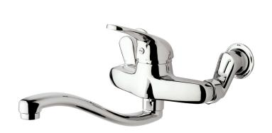
PRODUCT CODE FSX1 COLOUR/FINISHES Chrome All Pressures PRESSURE TYPE MIN. PRESSURE 35kPa MAX. PRESSURE 500kPa (As per NZ Building Code AS/NZ 3500.1) Low/Unequal 5 Star; 6L/min **WELS RATING** Mains 5 Star; 6.5L/min MAX. TEMPERATURE 65°C PLUMBING CONNECTION 15mm Mixer Handle - FORPT21 REPLACEMENT PART/S Cartridge – 40mm FORPT22 Spout - FORPT193 CERTIFICATION Watermark
