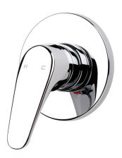
LT300 PRODUCT CODE COLOUR/FINISHES Chrome All Pressures PRESSURE TYPE 35kPa MIN. PRESSURE MAX. PRESSURE 500kPa (As per NZ Building Code AS/NZ 3500.1) 65°C MAX. TEMPERATURE 15mm PLUMBING CONNECTION FACEPLATE DIAMETER 115mm **EXCLUSIVE TO** Mitre 10 Cartridge – 40mm FORPT22 REPLACEMENT PART/S Faceplate - FORPT192 Lever - FORPT164
