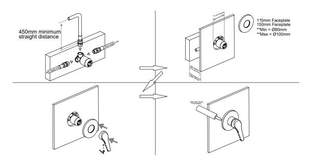
Plumbers Note: Do not pressure test this mixer under static pressure.
