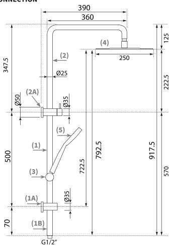
\*FOR PRESSURES EXCEEDING 500kPa INSTALL A PRESSURE
